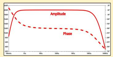
**Top Left:** Spectral density of the BHEMA sensor noise compared to 3-axis fluxgate magnetometer used in other BHEM probes. **Top Right:** BHEMA sensor response as a function of frequency. It behaves as a magnetometer between 0.2Hz and 25kHz. **Lower Right:** Field test comparison BHEMA vs Fluxgate. Signals from transmitter and powerlines clearly visible in the BHEMA data are overwhelmed by the noise of the fluxgate sensor.
