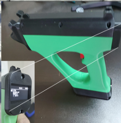
Handheld orientation tool using precision IMU.
