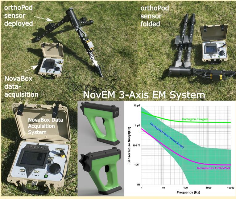
Channels: 3 differential Data Rate: 50,000 Timing: GPS (5us) Input : 200k-ohm Bandwidth: 1Hz-25kHz Weight: 1.7Kg
